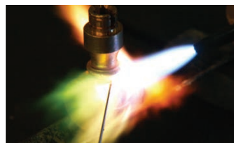
Brazing of a brass component
